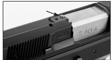
A loaded-chamber indicator pin atop the CZ 97's slide (arrow) is raised for visual or tactile inspection when a round is in the chamber.
